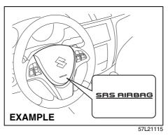
The driver's front air bag is located behind the center pad of the steering wheel and the front passenger's front air bag is located behind the passenger's side of the dashboard. The words "SRS AIRBAG" are molded into the air bag covers to identify the location of the air bags.
